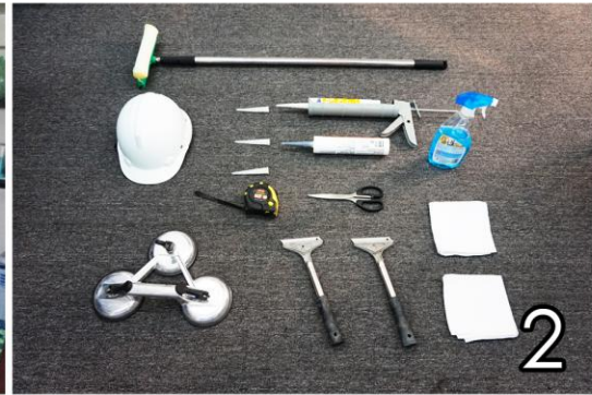
PREPARATION Silicone gel, Suction equipments for glass, Measuring tape, Scissors, Ruler, Soft cloth, Helmet, Wall scraper.
